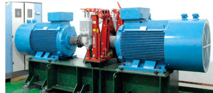
High power motor towing platform
