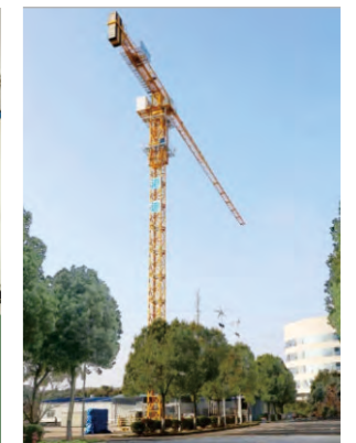
Tower crane test platform
